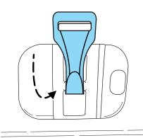
5. Tighten the child safety seat tether strap according to the manufacturer's instructions.
